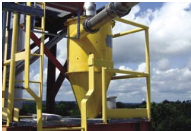
Cyclone clad with Conforma Clad® infiltration brazed tungsten carbide wear protection.
