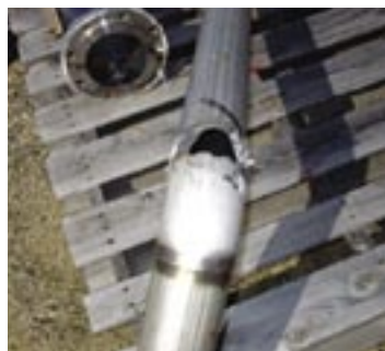
Elbow and pipeline blowouts were common before Solvay installed Conforma Clad® conveyance components.
