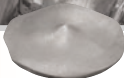
KenCast-protected VSI crusher center feed disk, above, and worn disk without KenCast, right.
