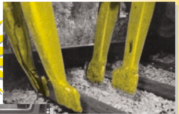
Railroad tamping tool with KenCast protection.
