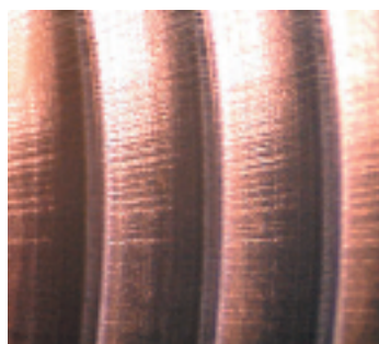
The threads on the left were cut by a Greenfield helical thread mill, while the threads on the right were cut by a competitor's conventional thread mill. Notice the chatter on the competitor's workpiece. The helical tool was so quiet, the operator wasn't sure it was cutting!
