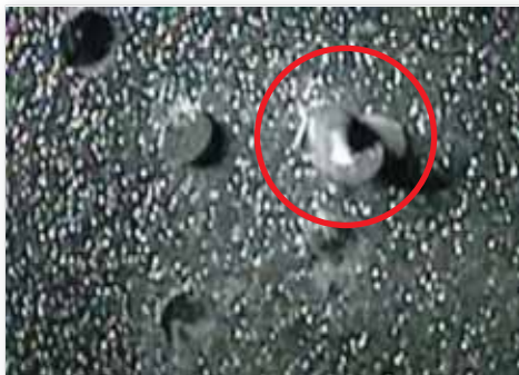
High-speed camera capture of breakout/delamination when hand-drilling in CFRP. Look closely for the extent of delamination prior to drill exit.
