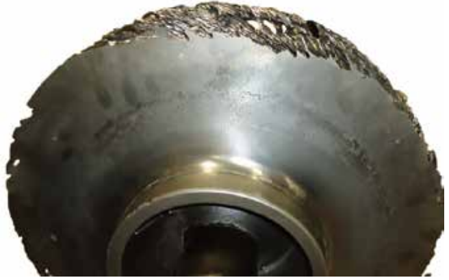
Pump impeller after 13 months without Conforma Clad protection
