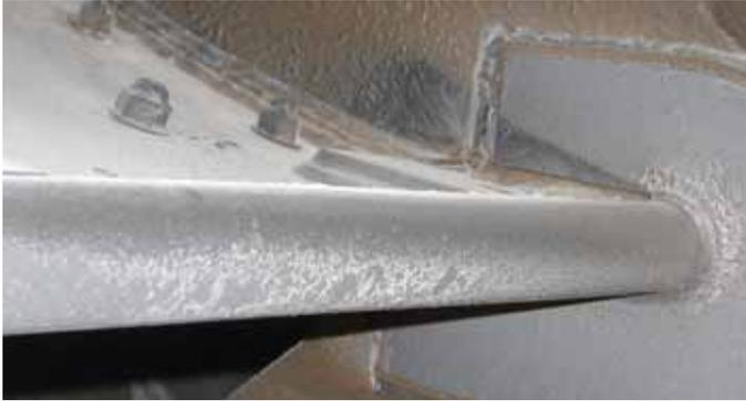
Kennametal's Conformal Clad™ tungsten carbide claddings have been cited by the Electric Power Research Institute as the most resistant of approximately 30 materials evaluated in fly ash erosion tests.
